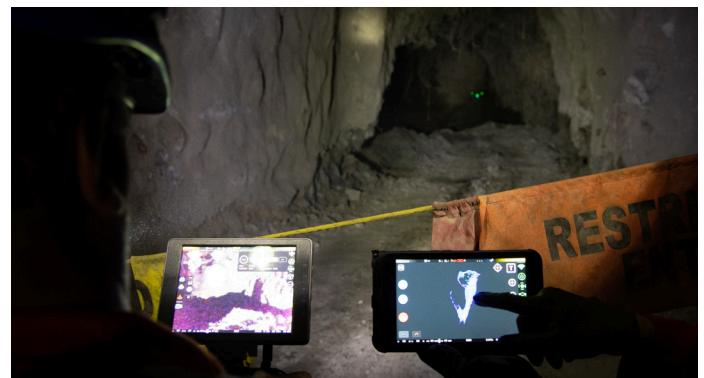
Remote inspections using Hovermap keep Kidd Operations personnel away from hazards.
