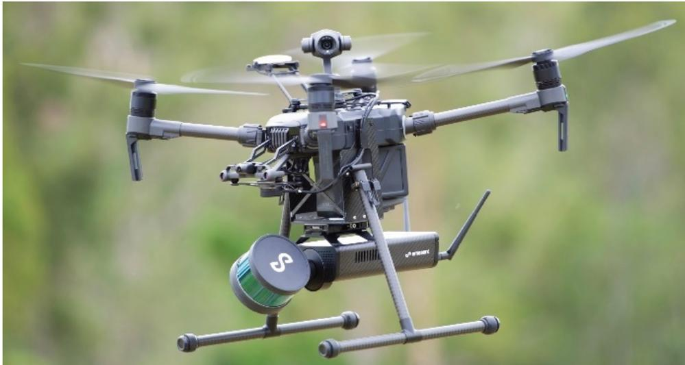
Figure 4 LiDAR system mounted onto a DJI Enterprise M210 Drone (Jones et al. 2020)
