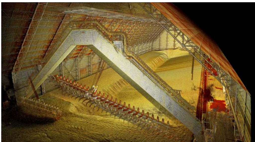
Example inspection and as-built capture of a 'buffer' facility at a mine in South Africa.
